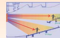
Beam splitting point: At the center point of all the transducers in a single stack.
